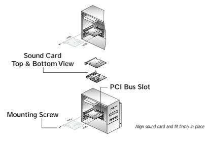
Use the screw from the slot cover to secure the sound card to the frame of the computer chassis, but do not over-tighten. Securing the card assures proper grounding.
